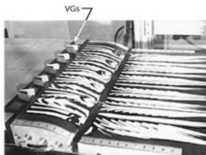
(b) 0.8 \delta -high vane-type counter-rotating VGs at 6 h upstream of baseline separation.
